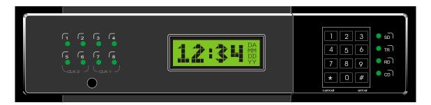
Your Master contains a lithium battery to keep the correct time when power has stopped due to an outage or the internal on/off switch. Once AC power resumes, your Master will calculate how much time your clocks lost and will automatically advance them to the correct time (this feature does not support Clock Types 14, 15 or 24).
