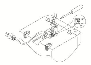
3 Insert wires into Terminals while pushing upper part of Terminal Block with screwdriver, then tighten both screws of cable clamp.
