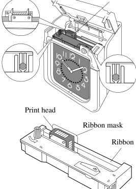
1 Unlock the unit. While holding down the panel open buttons at both sides of the unit, lift the panel cover away from you.
