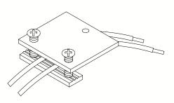
2 Feed wires through clamp. Do not tighten clamp screws.
