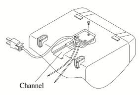
4 Fold down Cover Plate and secure with screw. Route Power and Bell wires through Channel in base of clock.
