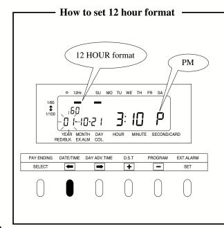
When you want to apply 12 hour format both on LCD time and printing format on the time card, select 12 hour format first as described below.
