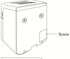
1 Unscrew the screw that holds the lid of the battery compartment in the lower right-hand corner of the back of the unit.
