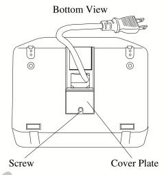
1 Unscrew the screw fixed on the bottom of the unit to remove the cover plate.
