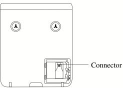
2 Insert the battery connector into the compartment connector to install the battery.
