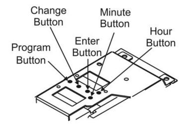
The **PROGRAM** button is used to enter and exit the Program Mode. If a program step is in the process of being changed when this button is pushed, the new information will not be saved.
