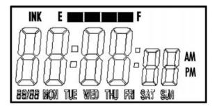
The PIX-28 calculates the ink capacity of the ribbon cartridge from the number of imprints made. As the ink capacity decreases, the bars in the gauge will disappear. If the ribbon reaches below 25% capacity, the "E", "F" and "INK" characters will blink until the ink counter is reset.
