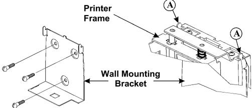
Securely mount the PIX mounting bracket on the wall using three #10 wood screws or equivalent. 4. Place the PIX-28 on the mounting bracket by sliding the top tabs into the slots on each side of the case. Push the PIX-28 back and down against the mounting bracket until the PIX-28 snaps into place. Be careful not to pinch the power cord with the bracket. Installing the cover will secure the PIX-28 to the mounting bracket.
