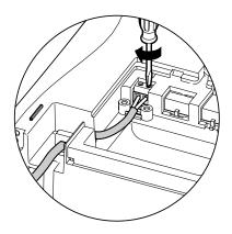
Insert Wires/Tighten Screws/Tuck Cord
