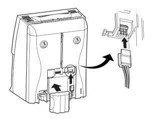
**Position Battery/Attach the Connector**
