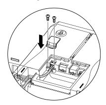
**Secure Wire Clamp with Screws**
