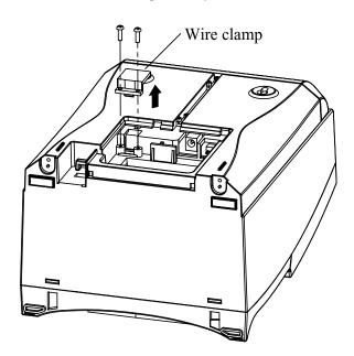
**Remove Two Screws Holding Wire Clamp**
